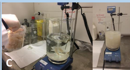
C: Pepsin digestion of rehydrated stockfish was used to assess the viability of nematodes.
